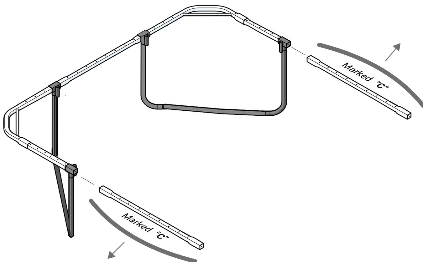
En: The slightly convex side should point outwards
